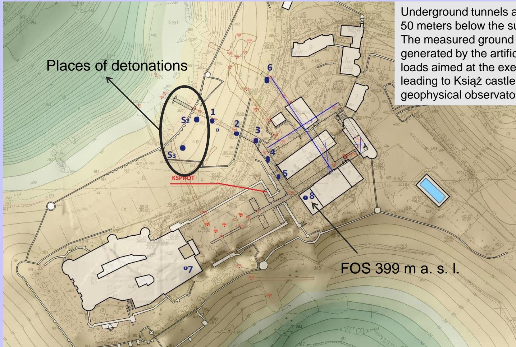
Underground tunnels are located at the level of -50 meters below the surface of the castle. The measured ground rotational movements were generated by the artificial explosions by dynamite loads aimed at the execution of tourist tunnels leading to Książ castle in near field of the geophysical observatory.
