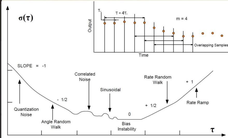
AV is a method of analysing a sequence of data in the time domain, to measure the frequency stability of oscillators.
