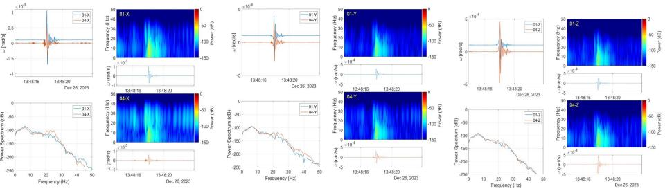
Correlation of about 95% for the X axis, about 99% for Y axis, and about 99% for the Z axis
