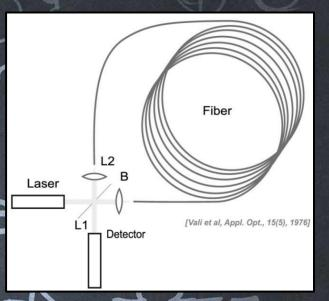
Sagnac effect shows the difference between phase of two beams propagating around closed optical path, in opposite direction when this path is rotating with rotational rate  $\Omega$ . In a fibre-optic implementation the rotation rate  $\Omega$  is expressed by induced phase shift  $\Delta \phi$  as:
