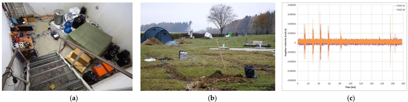
**Figure 11.** “Rotation and strain in Seismology: A comparative Sensor Test”, which took place in Geophysical Observatory Fürstfeldbruck, Germany: (a) the gathered rotational sensors in the bunker, (b) view of the test field during sensors installation, and (c) the data recorded by FOSREMS (type FOS5-01,-02) on the 19 November 2019.
