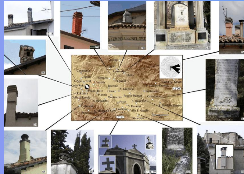
Map of the sites of observation of rotational effects and examples of rotations after 2009 L'Aquila earthquake [Cucci, L. & Tertulliani, A.. (2011), BSSA, 101, 1109-1120]
