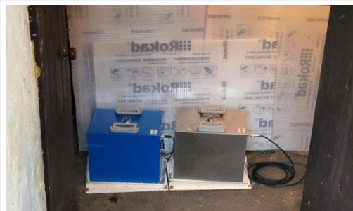
Field test in the Kampinos Nature Park by a pair of FORSs (FOS6-01 and FOS6-04)
